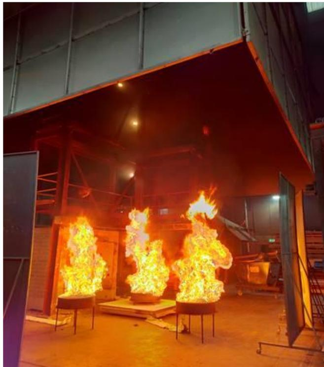
Figure F8. View of the hood calibration with 3 heptane pans
