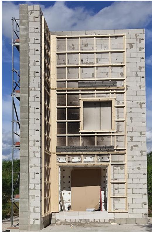
*Figure 4.2. Specimen without the timber cladding at ÉMI's laboratory. Additional cavity barriers and additional support for the cladding. Open cavity at the top.*
